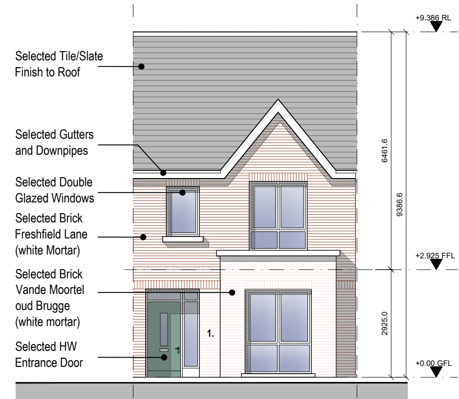
Type B1.2 Front Elevation Scale 1:100
