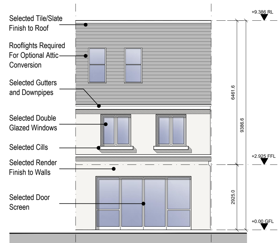
Type B1.2 Rear Elevation Scale 1:100
